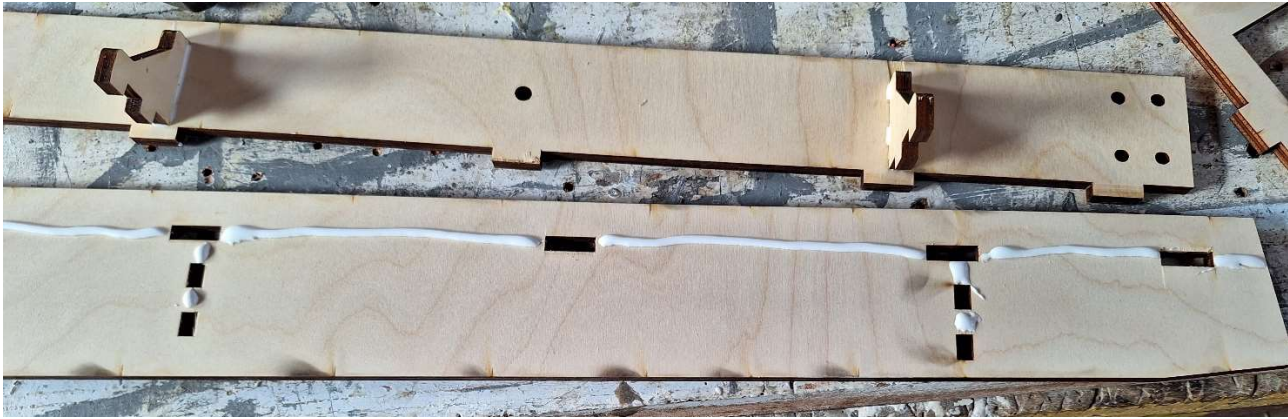
Fig 5 Glue beads on main face and stiffener assembly ready to fit
