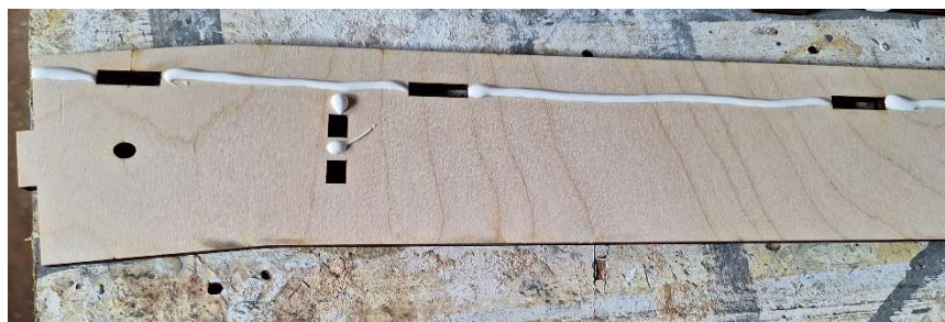
Fig 4 Glue position on main face
