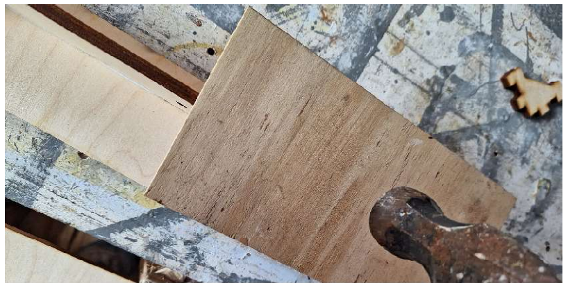
Fig 6 Tapping with hammer on scrap wood to protect the stiffener edge
