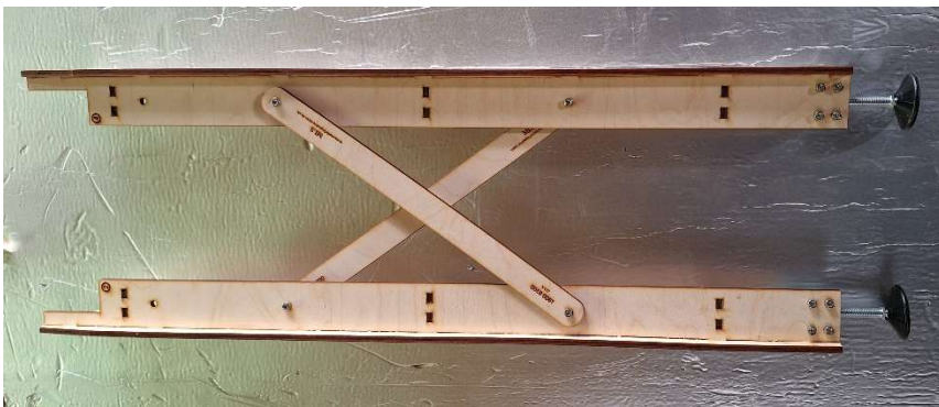
Fig 8 Assembled leg set with diagonal braces
