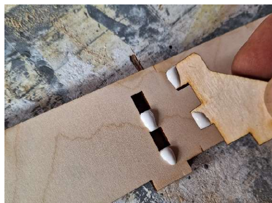
Fig 1 Glue location for triangle strengtheners
