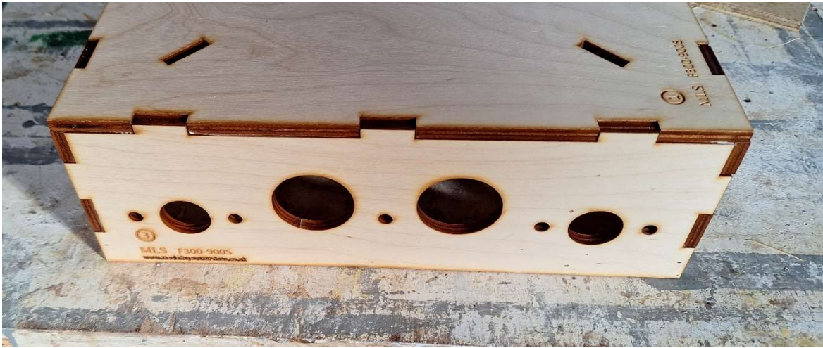
Fig 6 End piece fully home into baseboard top and side stringers
