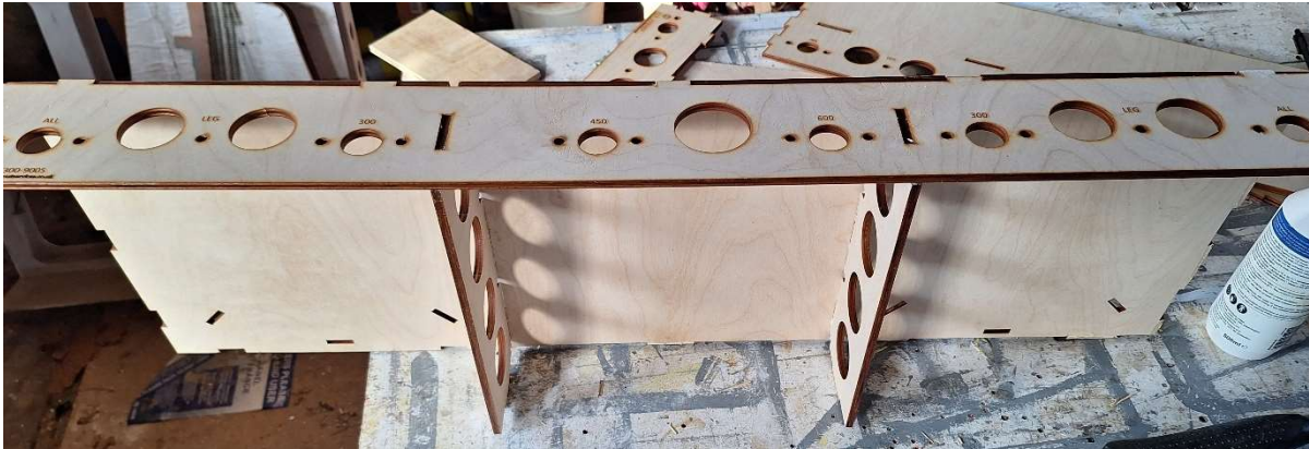
Fig 3 Side stringer fixed
